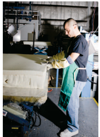
Above, a close look at the Tencel fabric with ultrasuede piping. Below, a worker positions a layer of latex foam into place.
